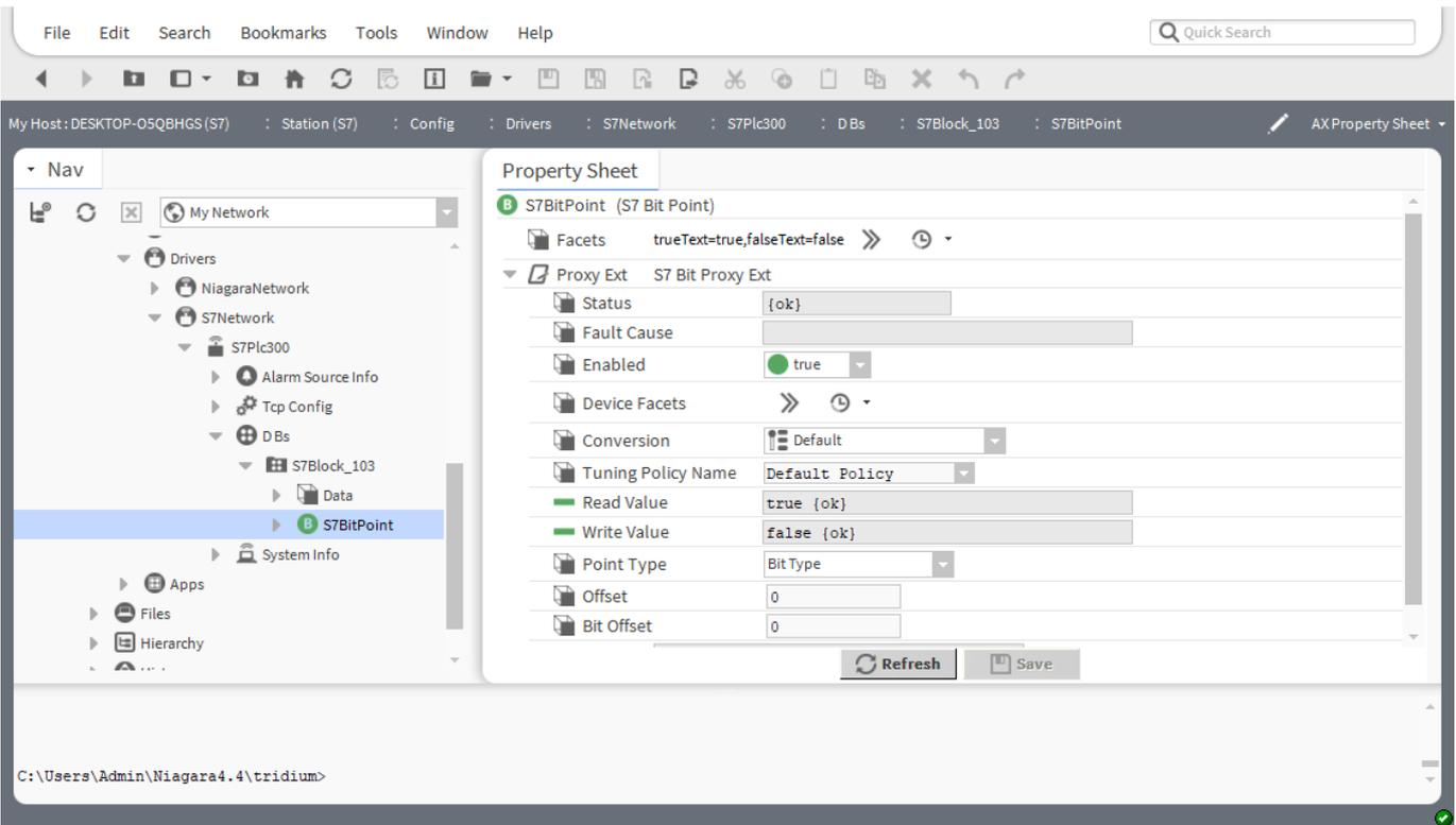
Figure 21: Set bit offset in the byte
