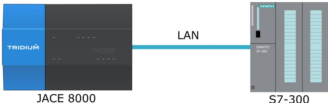
Figure 3: Diagram of connection to JACE 8000
