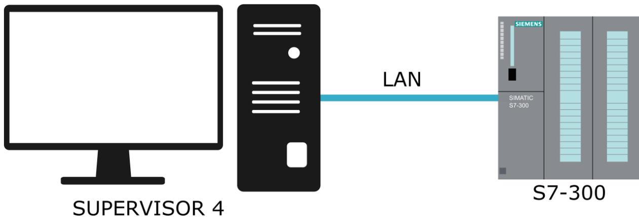
Figure 2: Diagram of connection to Supervisor 4
