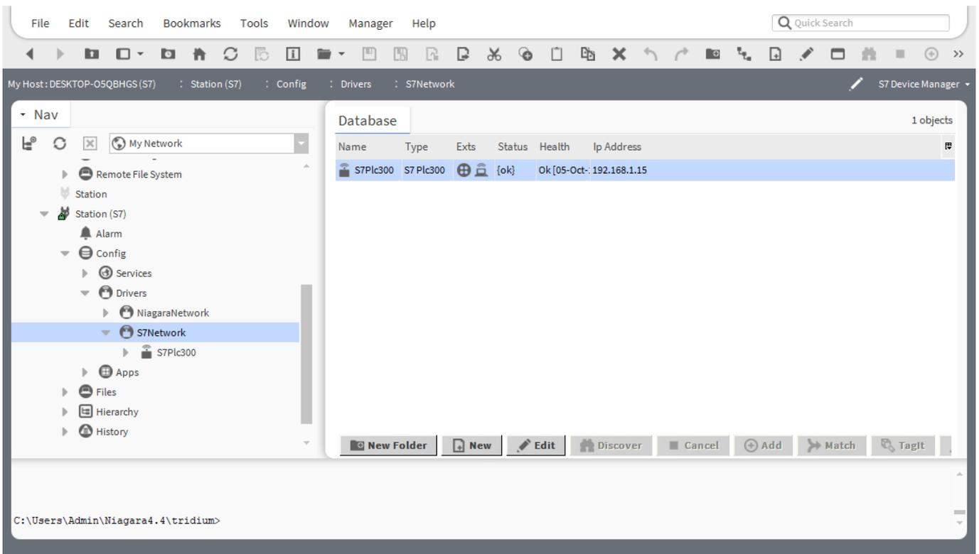
Figure 13: Health parameter of device should read ok
