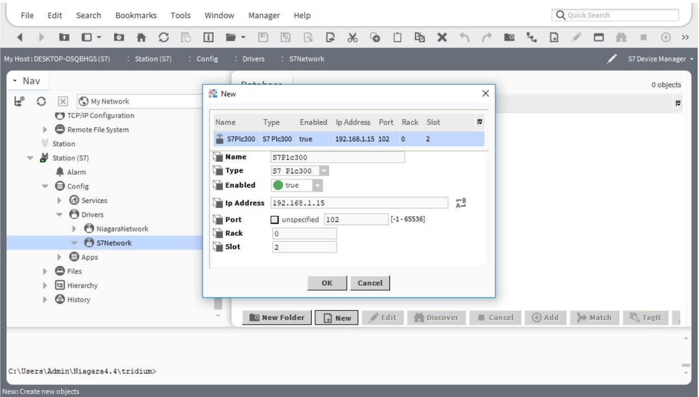
Figure 10: New S7 Device configuration menu
