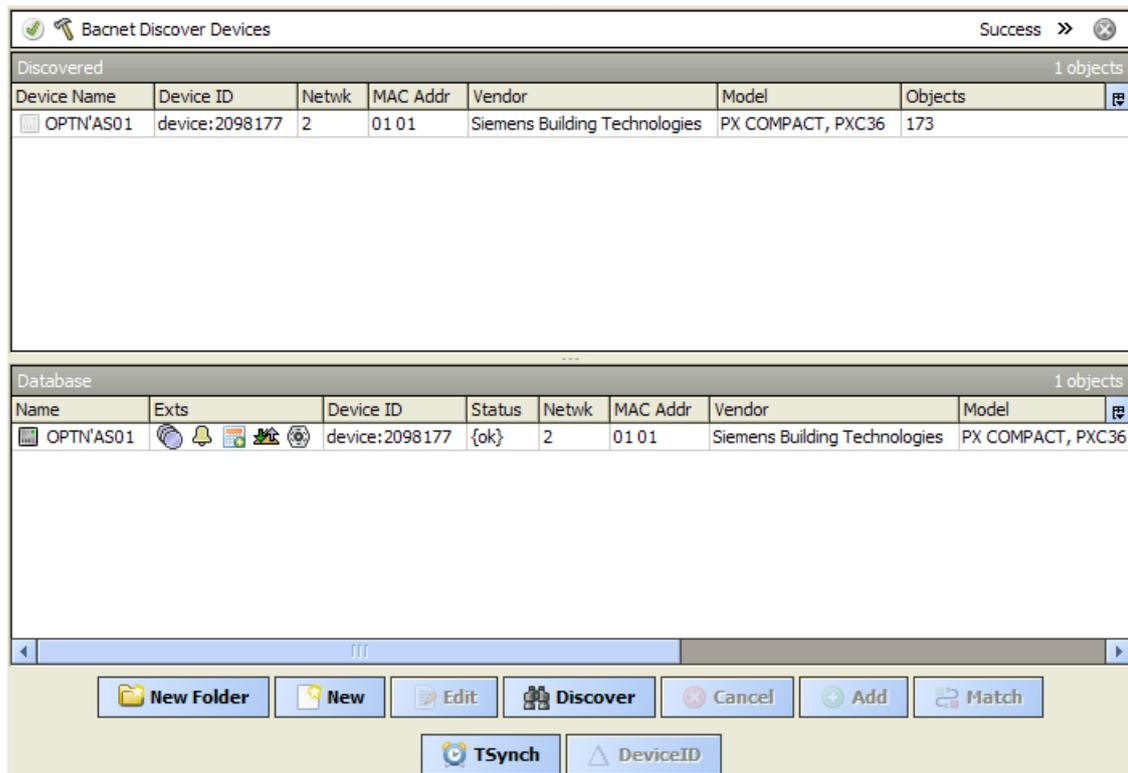
16. Add the devices by drag`n`drop or by pressing **Add** button. Select **DesigoDevice** (not **BacnetDevice**) type for added devices.
